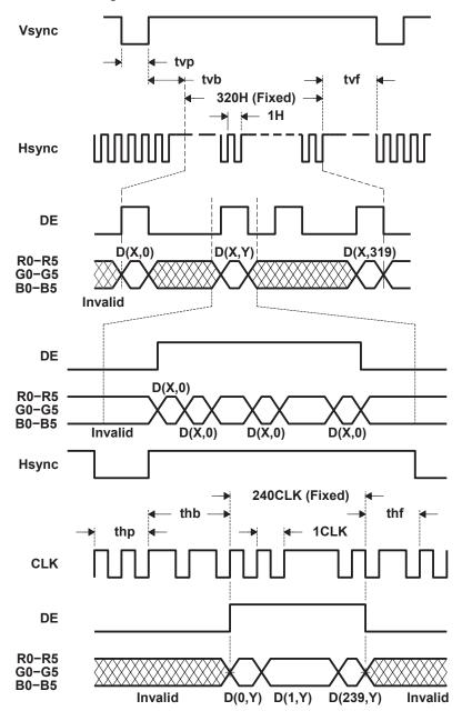
Figure 3. Data Enable Signal Timing Requirements
