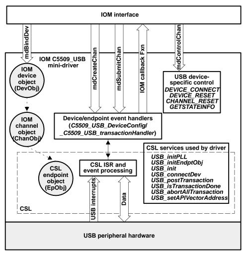
Figure 2. USB Interfaces and Data Structures
