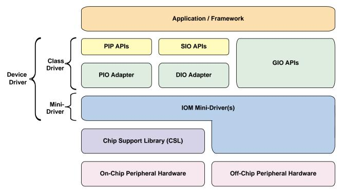
Figure 1. DSP/BIOS IOM Device Driver Model
