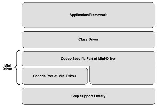
Figure 2. Codec Device Driver Partitioning
