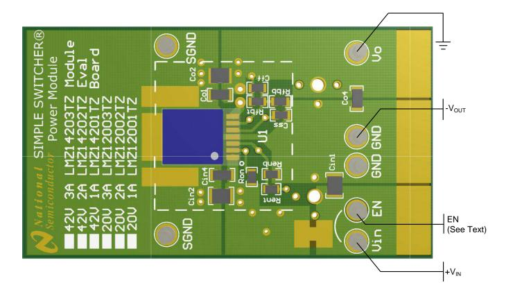
Figure 1. Evaluation Board Connections for Inverting Application
