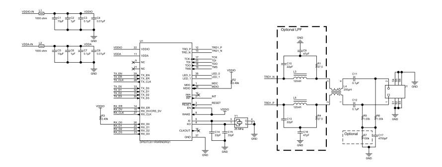
Figure 1. MII Schematic
