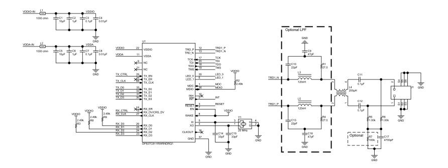
Figure 5. RGMII RX Shift Schematic
