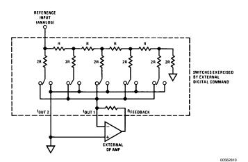
Details (Simplified) of CMOS DAC1020—Last 5 Bits Shown
