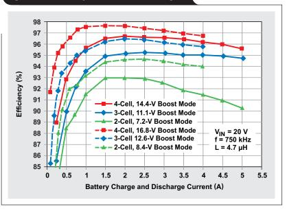
Figure 5. Efficiency of turbo-boost charger
