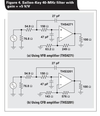
about a 540-MHz bandwidth. FilterPro realized the filters shown in Figure 4.
