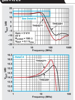
Figure 5. Sallen-Key filter responses with gain = +5 V/V
