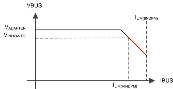
**Figure 1. Effective Input Current Limit Set by  $V_{INDPM}$**
