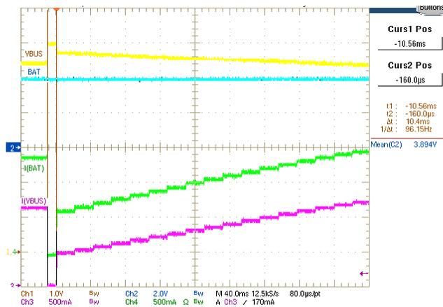
Figure 5. Forced ICO Detection With V(BAT) >  $V_{MINSYS}$
