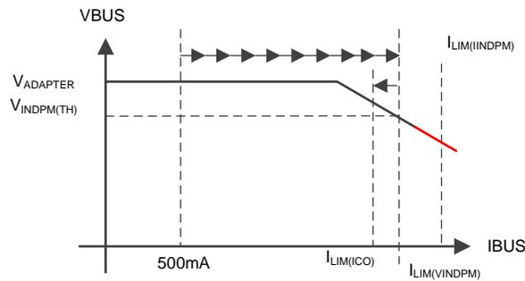
Figure 2. Graphical Representation of ICO During Operation
