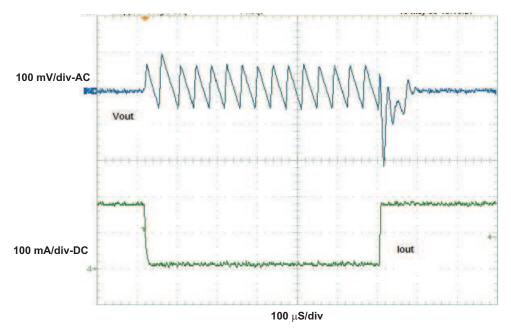
Figure 6. Figure 1 Circuit Transient Response With C6 = 1800 pF and R3 = 162 k $\Omega$
