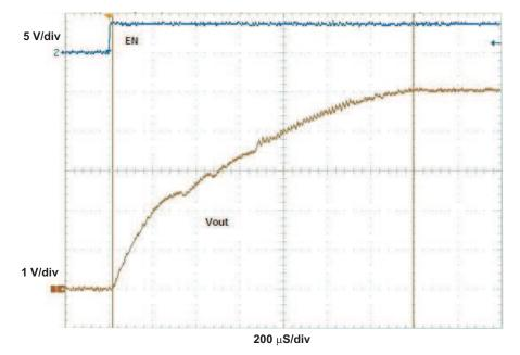
Figure 4. Figure 1 Circuit Soft Starting Into 50- $\Omega$  Load with C6 = 1800 pF and R3 = 162 k $\Omega$  – 1.379-ms Soft Start Time
