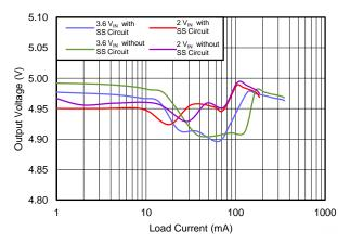
Figure 9. Load Regulation Effect of the Soft Start Circuit
