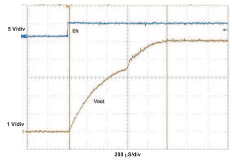
Figure 3. Figure 1 Circuit Soft Starting Into 50- $\Omega$  Load with C6 = 1000 pF and R3 = 162 k $\Omega$  – 971- $\mu$ s Soft Start Time
