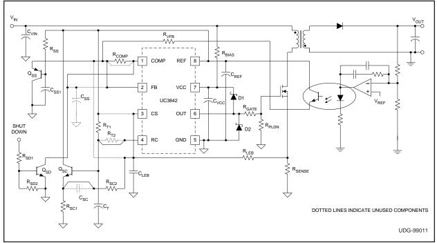
Figure 1. Isolated flyback converter using the UC3842.
