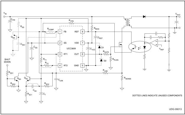
Figure 3. Isolated flyback converter using the UCC3809.
