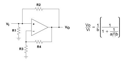
Figure 10. Model of High-Pass Sallen-Key Filter Above fc
