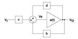
Figure 4. Gain-Block Diagram of the Generalized Sallen-Key Filter
