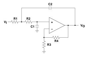
Figure 5. Low-Pass Sallen-Key Circuit
