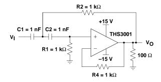
Figure 11. High-Pass Sallen-Key Filter Using THS3001
