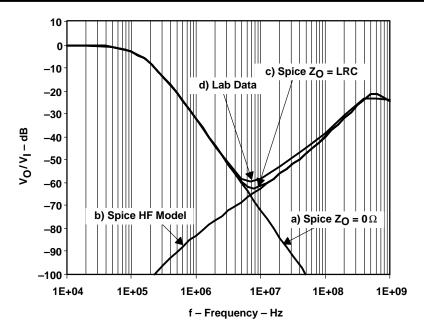
Figure 8. Effect of Output Impedance
