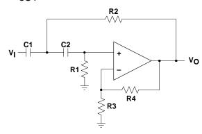
Figure 9. High-Pass Sallen-Key Circuit
