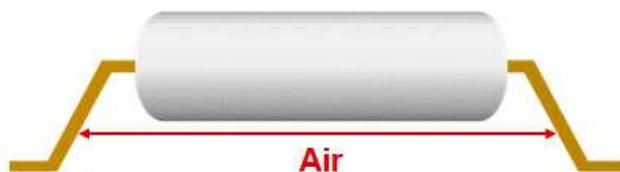
Figure 2. Clearance across a isolator package
