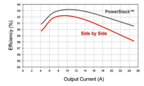
Efficiency @ V<sub>1</sub> = 12V, V<sub>GS</sub> = 5.0, V<sub>0</sub> = 1.3V,  $f_{SW}$  = 500kHz, L<sub>0</sub> = 0.3µH, T<sub>A</sub> = 25°C
