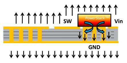
Figure 6: Optimal thermal path through grounded thermal pad of PowerStack Package.
