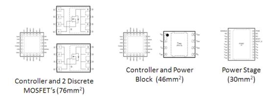
Figure 3: Board space savings for a typical circuit resulting from PowerStack.
