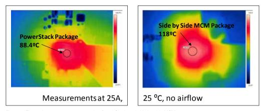
Figure 8: Thermal measurements comparing PowerStack and side by side MCM.
