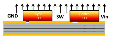
Figure 7: Limited thermal path through SW node and Vin node of side by side MOSFET's.
