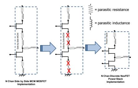
Figure 4: PowerStack delivers low parasitic losses to support high current levels and high switching frequency.
