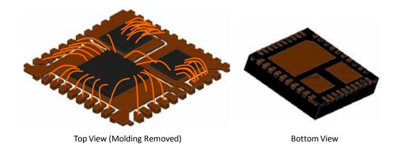
Figure 1: A side-by-side implementation of two MOSFETs with a controller IC
