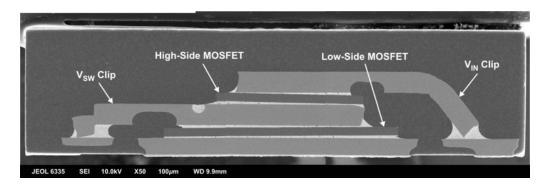
Figure 2: A cross-section of a device using a PowerStack package.
