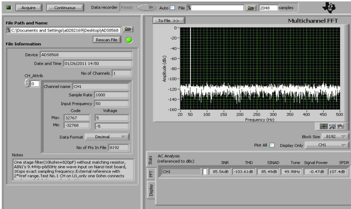
Figure 14. FFT for 1-KSPS Sampling Rate ( $V_s = -0.5$  dBFS)
