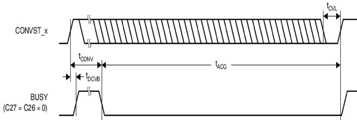
**Figure 3. ADS8568's Acquisition Time and Conversion Time**
