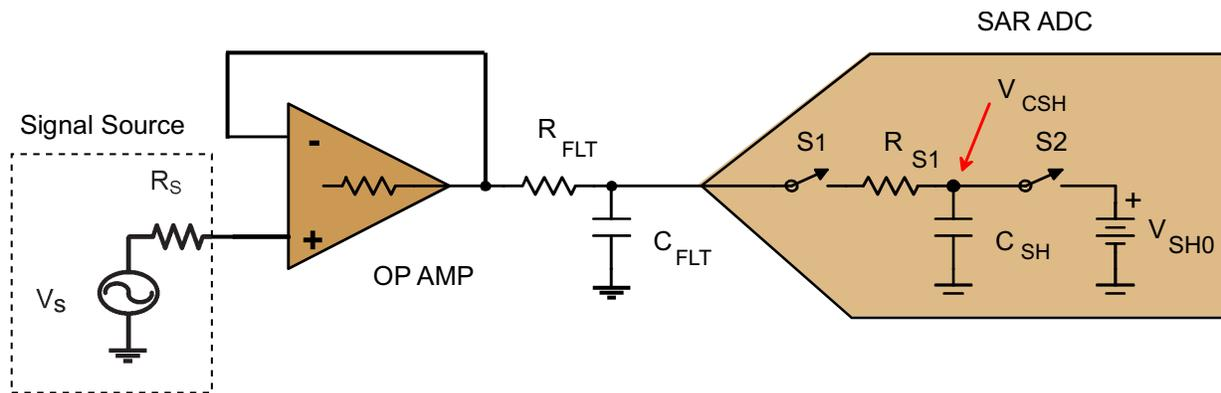
**Figure 1. Typical Driver Circuit for SAR ADC**
