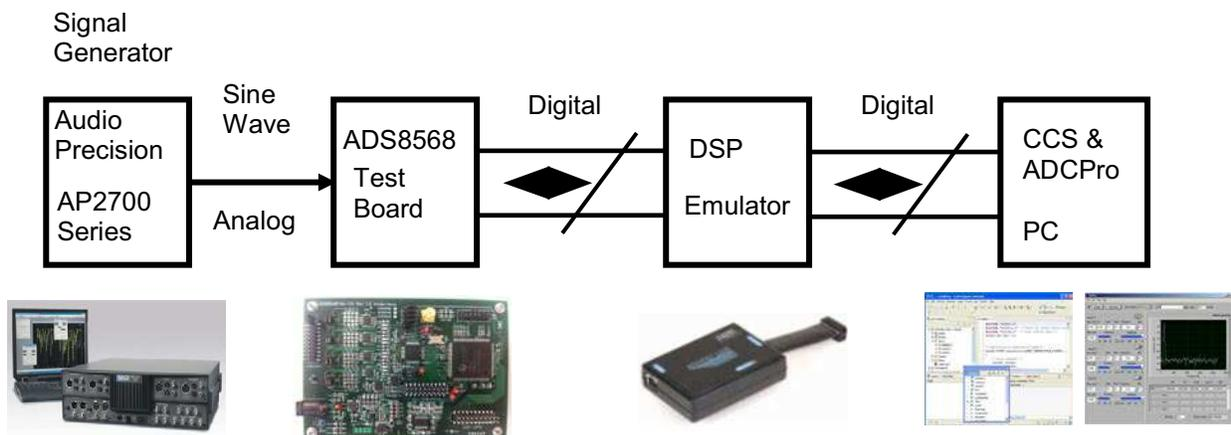
Figure 5. Performance Test System for the ADS8568 Circuit
