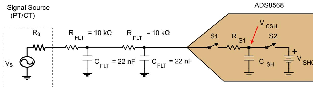
Figure 2. ADS8568's Driver Circuit Without a Front-End Amplifier
