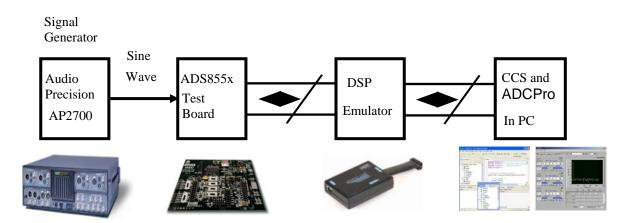
Figure 4. Performance test system for ADS8556 circuit
