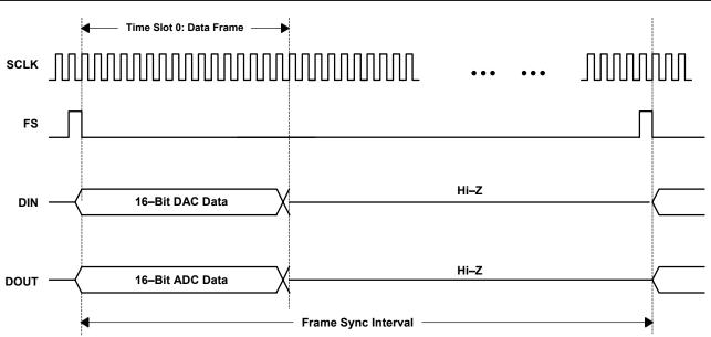
Figure 7. Turbo Continuous Mode Timing, Stand-Alone Slave
