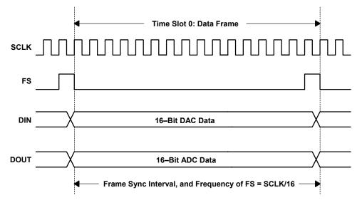
Figure 6. Standard Continuous Mode Timing, Stand-Alone Slave
