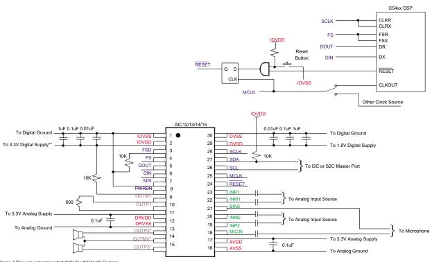
\* These 3 Pins are not connected (NC) for AIC14/15 Codecs \*\* To 1.1 ~ 3.6 Vdc Digital Supply for AIC13/15 Codecs.
