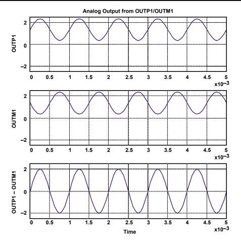
Figure 8. Single-Ended or Differential Signals at OUTP1/OUTM1
