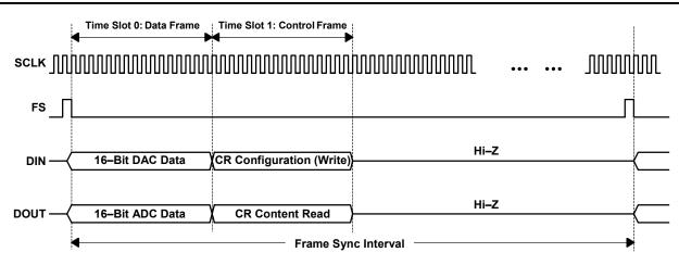
Figure 5. Turbo Programming Mode Timing, Stand-Alone Slave
