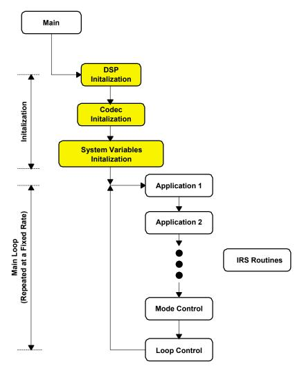
Figure 9. DSP/Codec Firmware Structure
