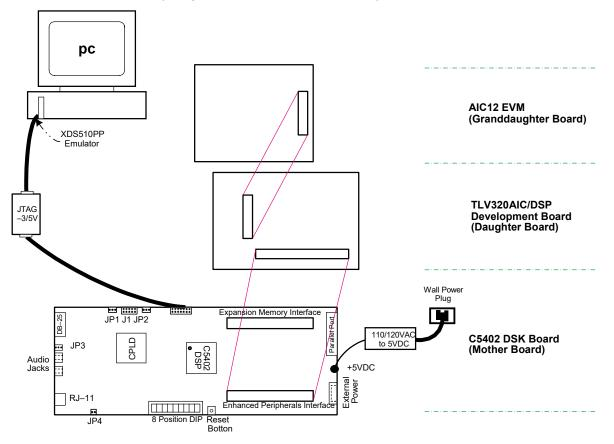
Figure 3. AIC/DSP EVM System Connection
