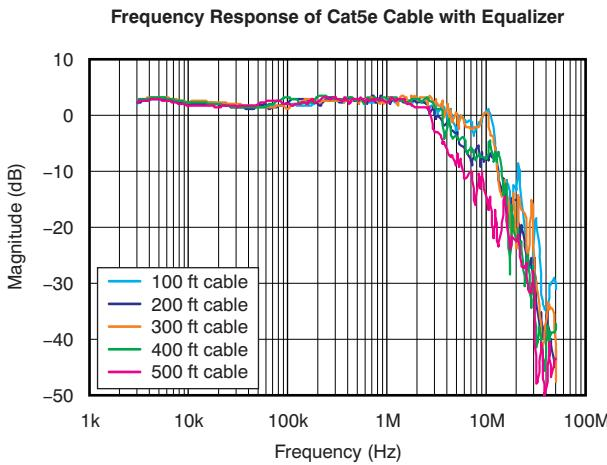
**Figure 8. Equalized AC Responses for Different Lengths of Cat5e Cable**
