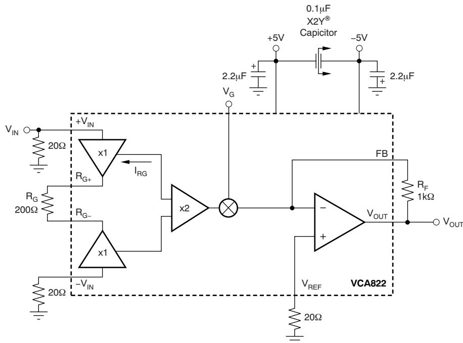
**Figure 2. VCA822 Internal Schematic**
