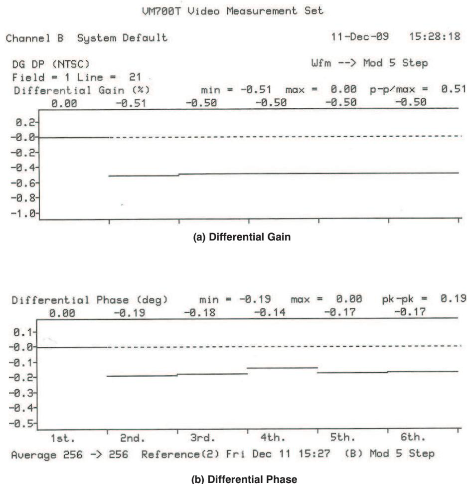
**Figure 9. Differential Gain (a) and Differential Phase (b) Measurements for 500ft Cat5e Cable**
