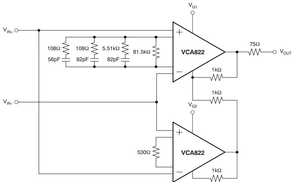
**Figure 3. Equalizer Circuit Using the VCA822**
