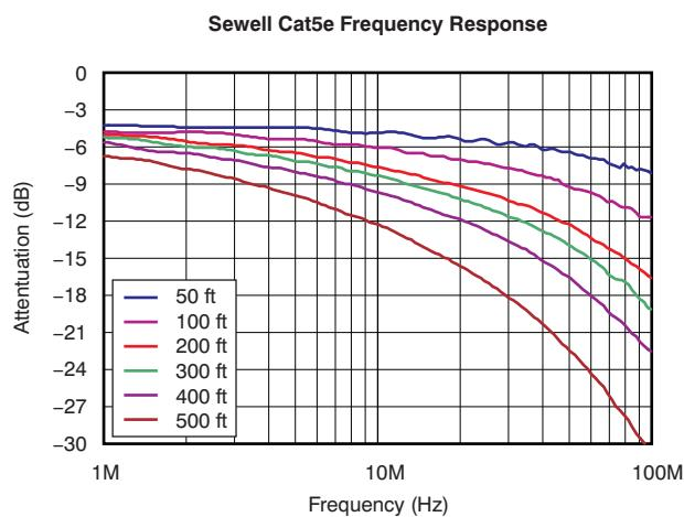
**Figure 1. Typical Attenuation Characteristics of Cat5e Cable**
