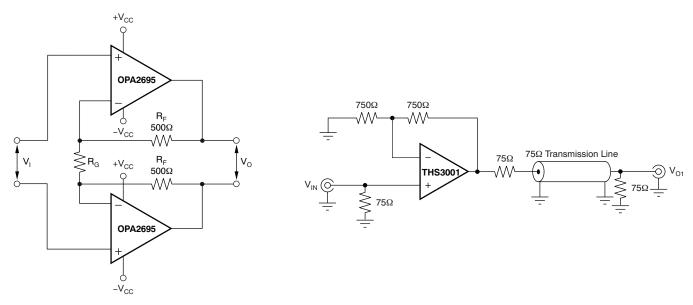
a) Typical Twisted-Pair Driver Cable Circuit
