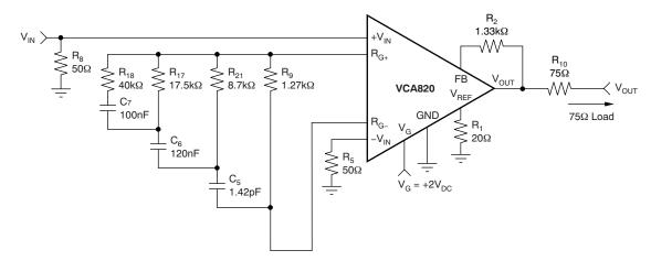
Figure 8. Equalizer Circuit for 100ft of Belden 1694F Coax Cable
