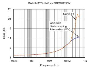
Figure 13. Theoretical Gain Matching to the Attenuation
