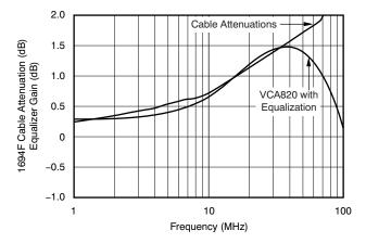
Figure 9. Cable Equalization and Cable Attenuation Comparison
