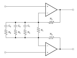
Figure 5. Differential Equalizer Circuit
