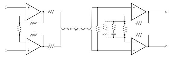
Figure 12. Proposed Tx and Rx Schematic
