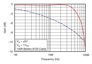
Figure 15. Measured Circuit Performance
