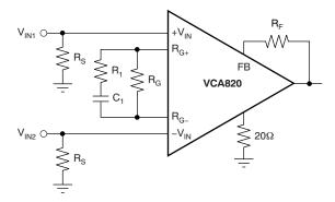
Figure 7. Differential Equalizer Circuit (VCA820)
