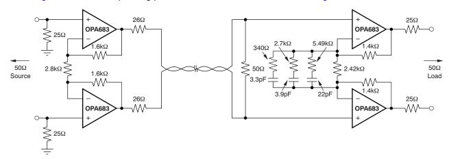
Figure 14. Developed Tx and Rx Circuit with the OPA683
