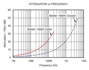
Figure 1. Attenuation vs Frequency for Cat5e and 75 $\Omega$  Coax Cables
