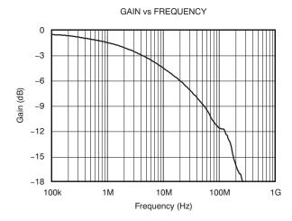
Figure 11. Belden 8723 Shielded Twisted-Pair Frequency Response
