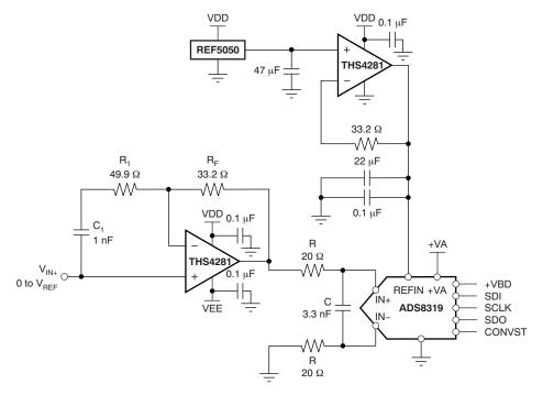
Figure 6. ADS8319: Driver Configuration
