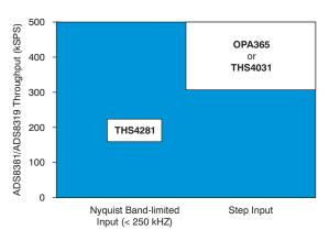
Figure 12. THS4281 Operating Region and Power Dissipation Comparison
