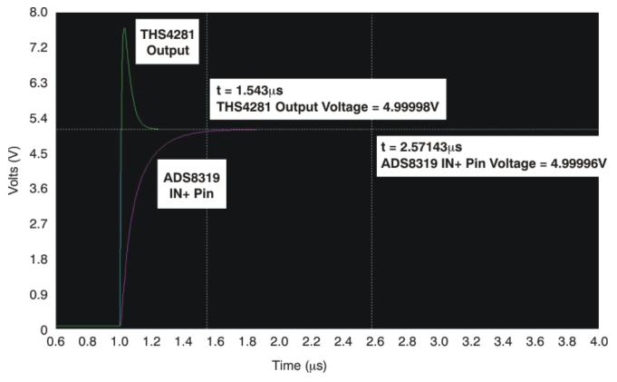
Figure 11. Step-Input Response for Circuit Shown in Figure 6
