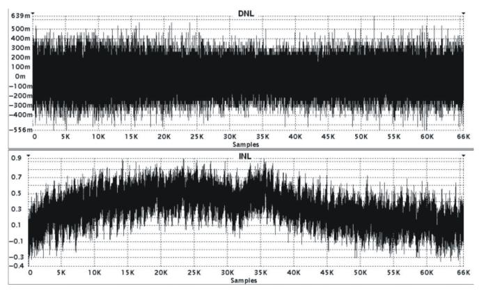
Figure 9. ADS8318: Typical Linearity Graphs (Single-Ended Configuration)
