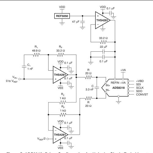
Figure 5. ADS8318: Driver Configuration for Unipolar Single-Ended Input
