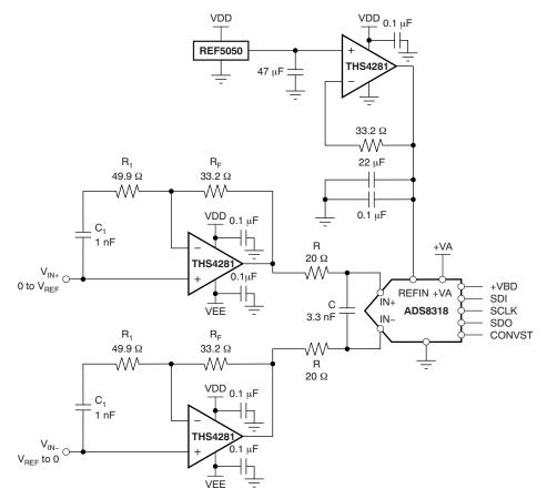
Figure 4. ADS8318: Driver Configuration for Unipolar Differential Input
