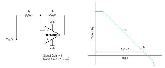
Figure 2. Reduced Feedback Factor Reduces Peaking
