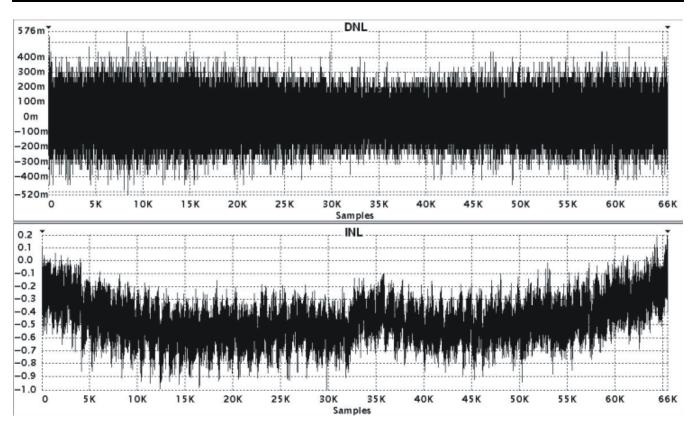
Figure 8. ADS8318: Typical Linearity Graphs (Differential Configuration)
