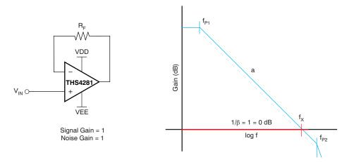
Figure 1. Open-Loop Gain vs Frequency (Generic Op Amp Response)
