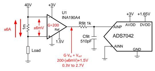
High-side current shunt monitor circuit to 3-V single-ended ADC
