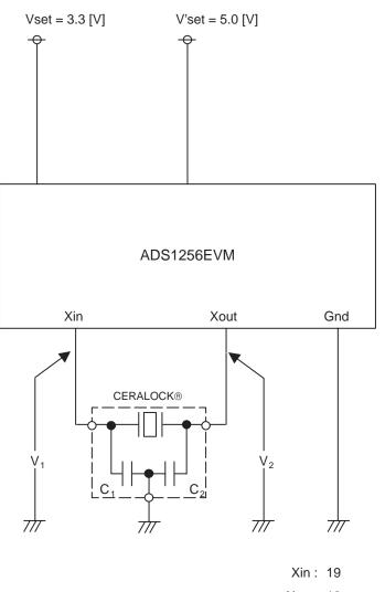
Xin : 19 Xout: 18 Recommended Value CERALOCK® : CSTCR4M00G53-R0 Vset = 1.5 to 3.6 [V] C1 = 15 [pF] (Typ.) C2 = 15 [pF] (Typ.) Ta = -40 to 85 [°C]
